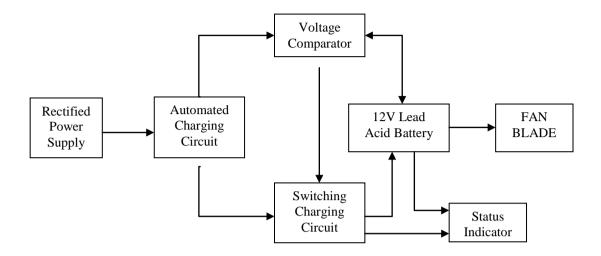
Figure 1: Block Diagram of the Rechargeable Electric Fan
