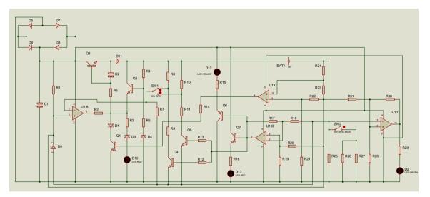
Figure 2: Automated Charging Circuit Diagram
